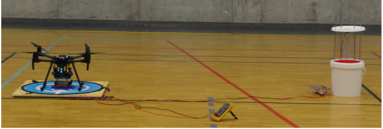
Fig. 5: Energy providing through UAV, complete set-up
