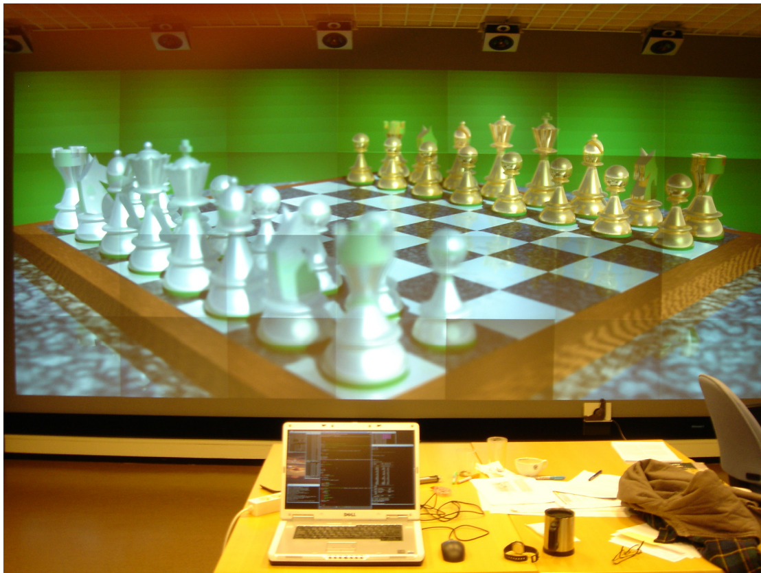
Figure 8. The completed image. For size comparisons, note that the portable computer on the table is a 17-inch notebook and that the display wall is about 3 meters from the table.
