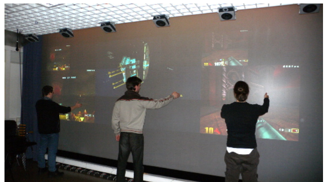
Figure 1. Two persons playing Q3A and one person playing Homeworld simultaneously on a 7x4 tile display wall. Q3A runs on 2x2 tiles to the left and right, and Homeworld on 3x3 tiles in the middle.
