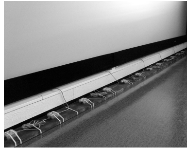
Figure 6. The image shows 12 of the 16 cameras mounted along the floor and looking at the ceiling.
