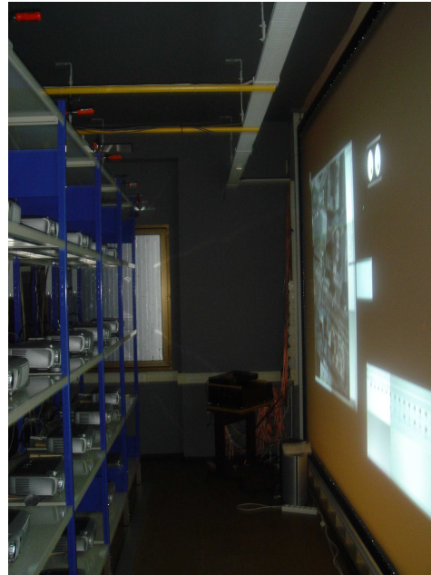
Figure 1.1: The projectors creating the display wall.
