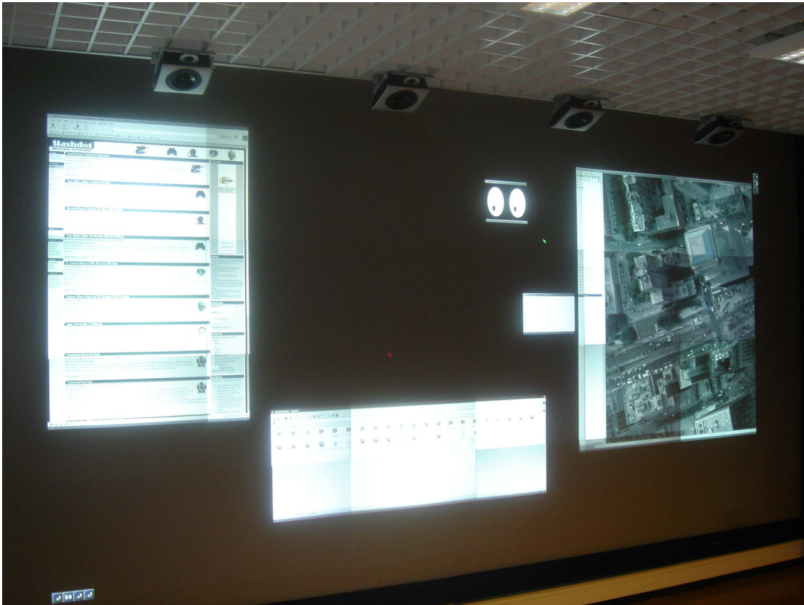
Figure 1.3: The display wall running the multi-cursor window manager and some applications.
