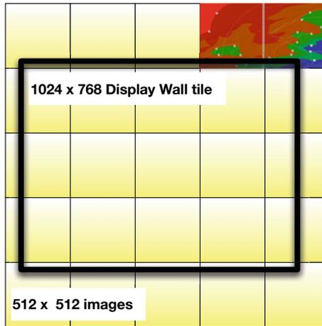
**Fig. 5.** Illustration of the parts needed for one tile of the display wall. Each image requested from the LDS is 512x512 pixels. Each display wall tile has a resolution of 1024x768 pixels. The WallGlobe will always use images with higher or equal resolution to the tile's resolution.
